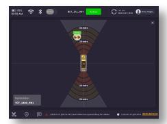
Collision Alerts to detect and alert miners and equipment in close proximity.
