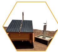
Base Station Positioned strategically for extended coverage (15-20km range)
